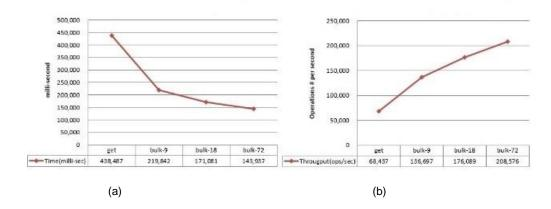
As seen from the timing graph (a) above, getting 30 M rows using simple get api would have taken us 420 seconds, which reduces to 149ms with 72 executor threads (Plotted on X-Axis) using the bulk get API. This is almost a 3X improvement! And as seen on the graph (b) the throughput went to 200K ops/s with 72 executor threads from 68k ops/sec using a simple get operation. That is again a **3X improvement**!
