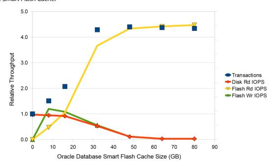
Figure 2: Relationship between Throughput and Disk and Flash I/Os
