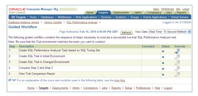
Real Application Testing was introduced in the 11g release of the Oracle Database, however, SQL Performance Analyzer is also available for previous releases of the Oracle Database. Consequently, SQL Performance Analyzer can be used to test changes in SAP environments even if there are no immediate plans to move to Oracle Database 11g Release 2.
