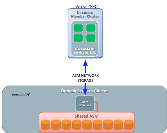
Figure 6b. ASM Network Attached Storage
