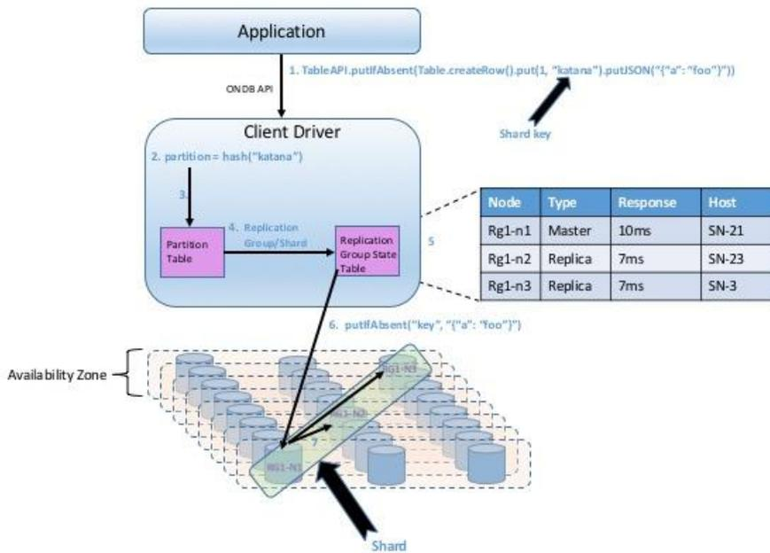
Figure 3 – Architecture - Oracle NoSQL Database – Write Request Flow
