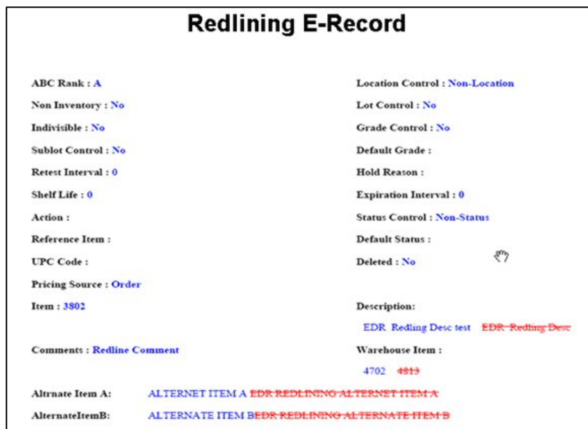
Figure 1: Redlining can show users, exactly what is changed in current transaction e-record
