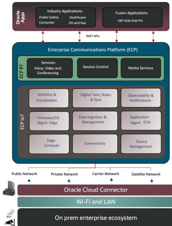
Image 1: Oracle Cloud Connector is the edge hardware within the Oracle ECP architecture, strategically extending secure and resilient connectivity, as well as cloud services, directly to locations where data is created and business operations occur.
