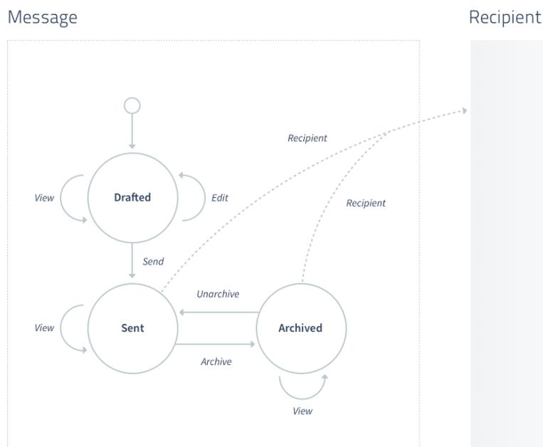
You may draw a finite state machine diagram to identify the states of your resources and discover the relations between resources. This state machine diagram will help to recognize what resources are actually needed. In addition, the finite state machine diagram helps you to understand how the API might be implemented.
