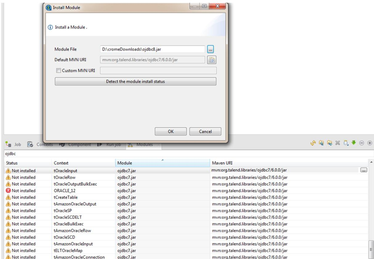
10. Once the ojdbc8.jar driver is loaded, you can now create a Metadata DB connection. Click Metadata → Database Connection → Create Connection.
