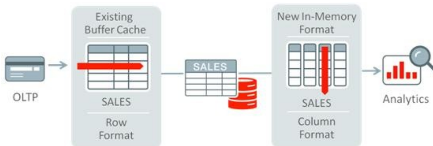
Figure 1: Dual format in-memory representation featuring new in-memory column store
