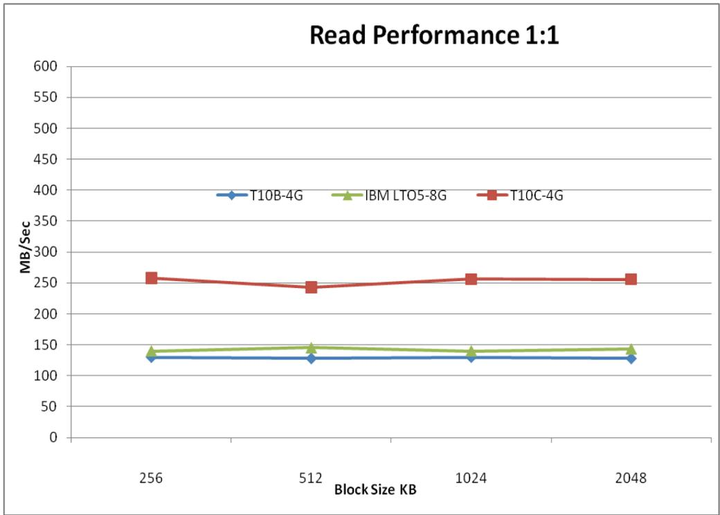
Figure 5: Read comparison at 1:1 compression ratio
