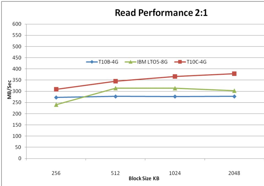
Figure 7: Read comparison at 2:1 compression ratio
