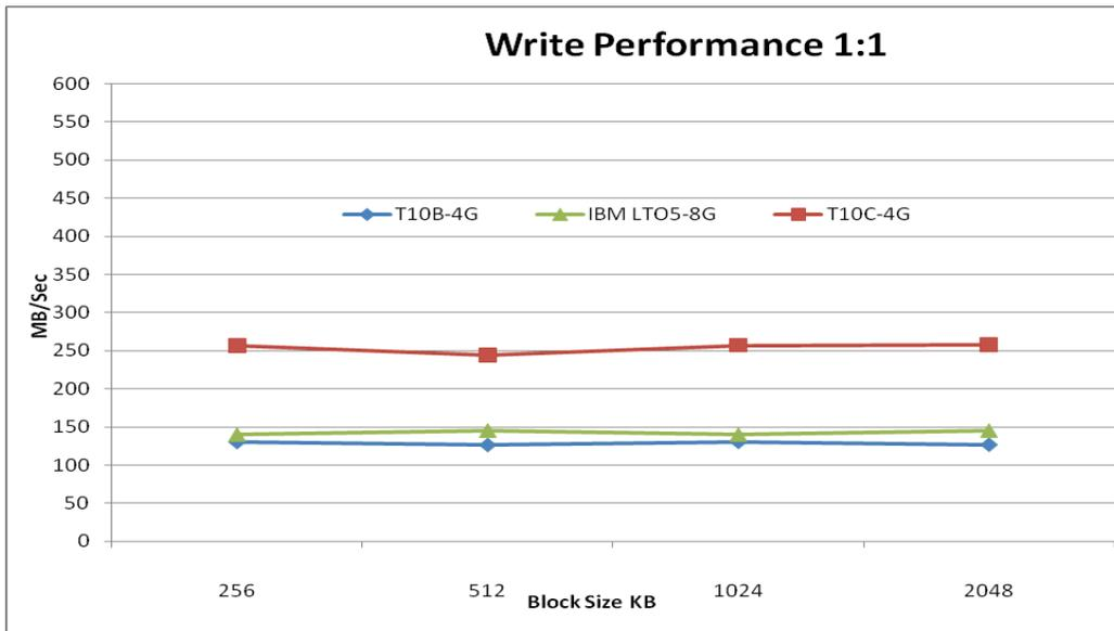
Figure 4: Write comparison at 1:1 compression ratio
