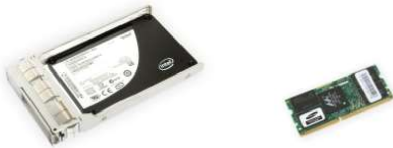
Figure 10. Solid-state drives (left) provide enterprise flash technology in a standard disk drive form factor. Oracle's Sun FlashFire technology (right) provides optimized performance in a considerably smaller form factor.
