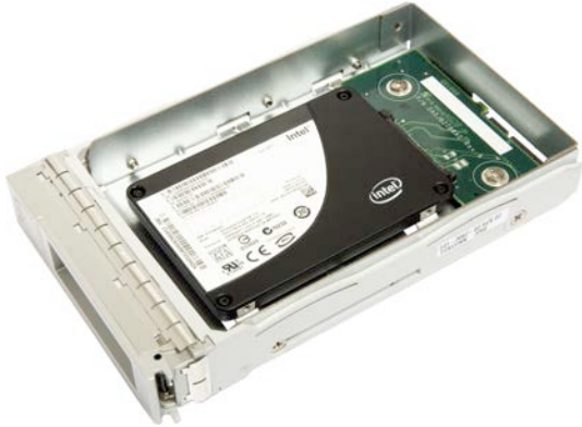
Figure 5. Sun Fire X2270 M2 solid-state drives—shown in the sample drive above—are effective and reliable solutions for enterprise storage.
