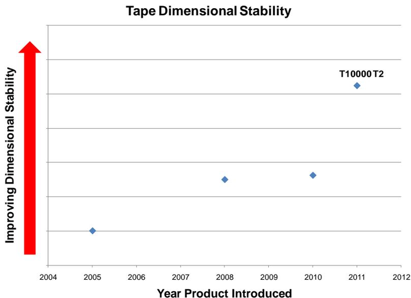
**Figure 2.** Tape dimensional stability is improving with new tape drive offerings. The StorageTek T10000 T2 tape media has the greatest tape dimensional stability. This is made possible through the use of aramid as the tape substrate.
