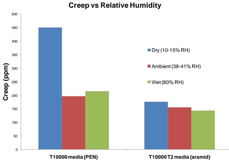
**Figure 4.** This data shows how changes in humidity can also influence tape dimension. Media using PEN substrates are affected more than the new, second generation of StorageTek T10000 media (T2), which uses aramid.
