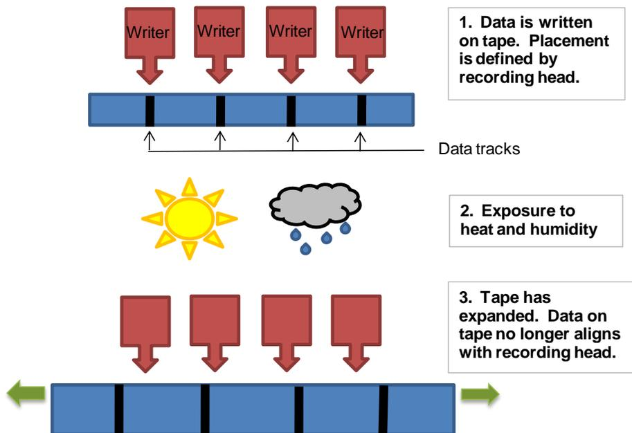
**Figure 1.** Small changes in the dimensions of the tape can affect the read back quality of data.
