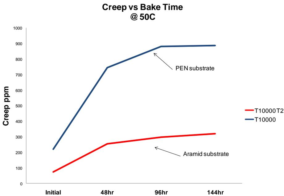
**Figure 3.** Magnetic tapes with a PEN substrate change width appreciably more than the newest magnetic tape offering from Oracle, StorageTek T10000 T2, for use with the StorageTek T10000C tape drive.
