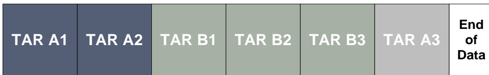
Figure 4: TAR A3 which is associated with TARs A1 & A2 is written at EOD
