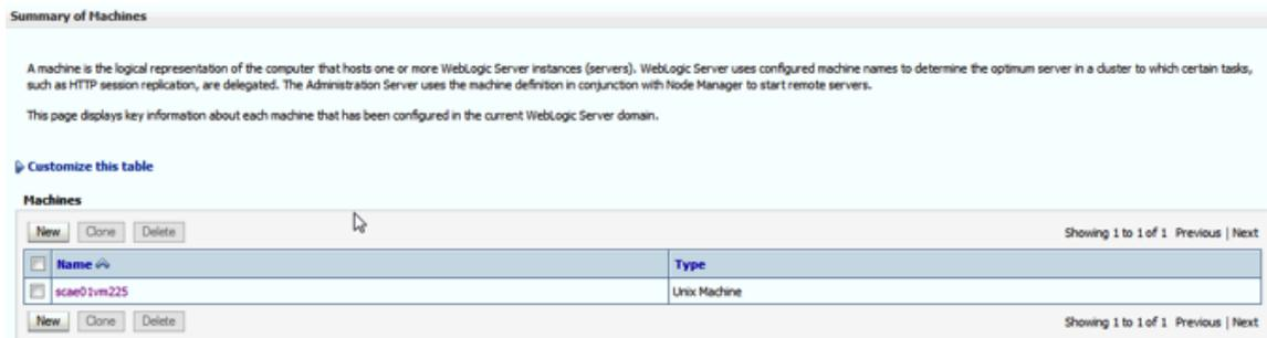
3. If no machines appear in the **Summary of Machines** page then click **New** to add the machine, using a Plain UNIX machine and the hostname, then check the Node Manager tab.
