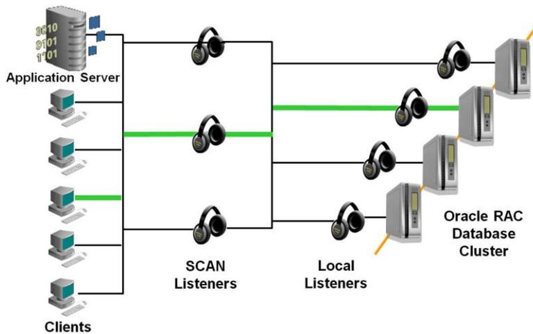
Figure 1: Connection Load Balancing using SCAN - Illustrated
