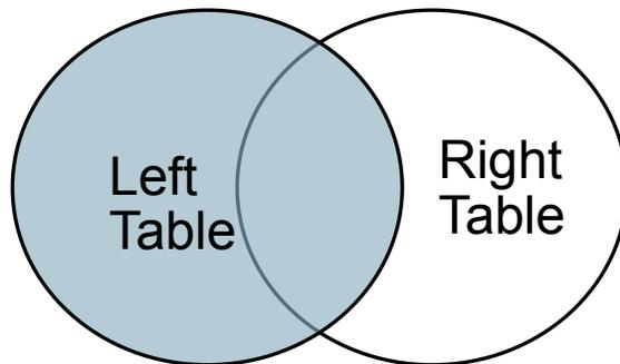
The above Venn diagram depicts the LEFT OUTER JOIN, with the shaded part showing what rows are returned. The intersection between two circles are rows that match in both tables, and the remaining part of the left circle are rows in the table that do not have any matching row in the right table. Hence, all rows in the left table are included in the result.
