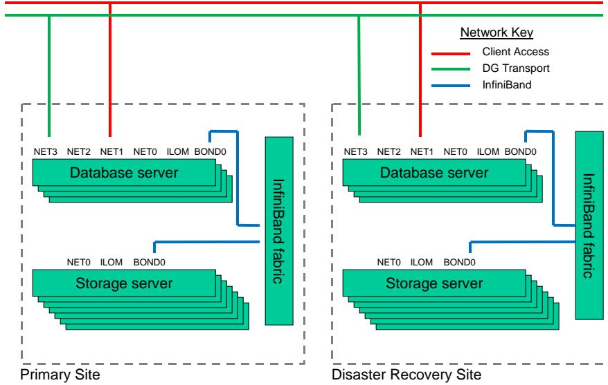
FIGURE 2, ISOLATE DATA GUARD REDO TRANSPORT FROM CLIENT ACCESS
