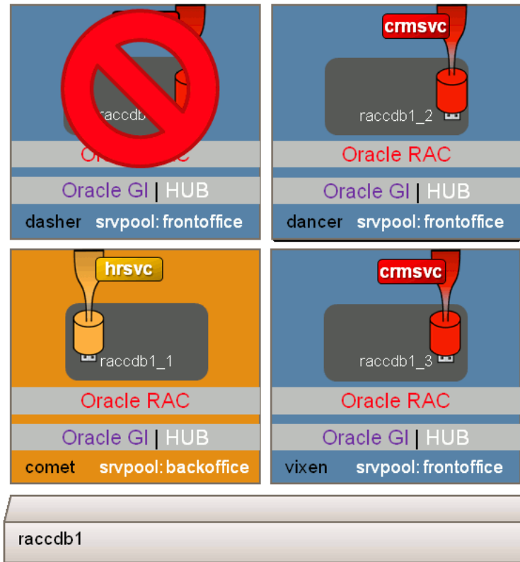
Figure 4: New Failover Policy-based Behavior
