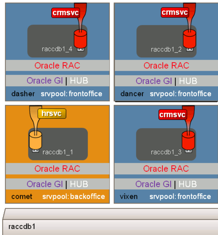
Figure 8: Server Pools Dynamically Sized to Meet Demand
