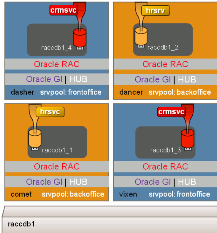
Figure 1: Example Cluster with Multitenant RAC database
