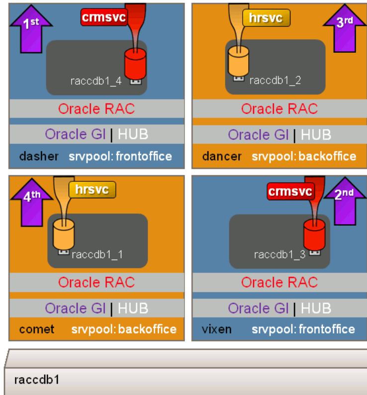
Figure 3: Service and Instance Start Order
