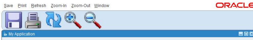
Figure 10 : smartBarHeight set to large and using 48x48 pixel images.
