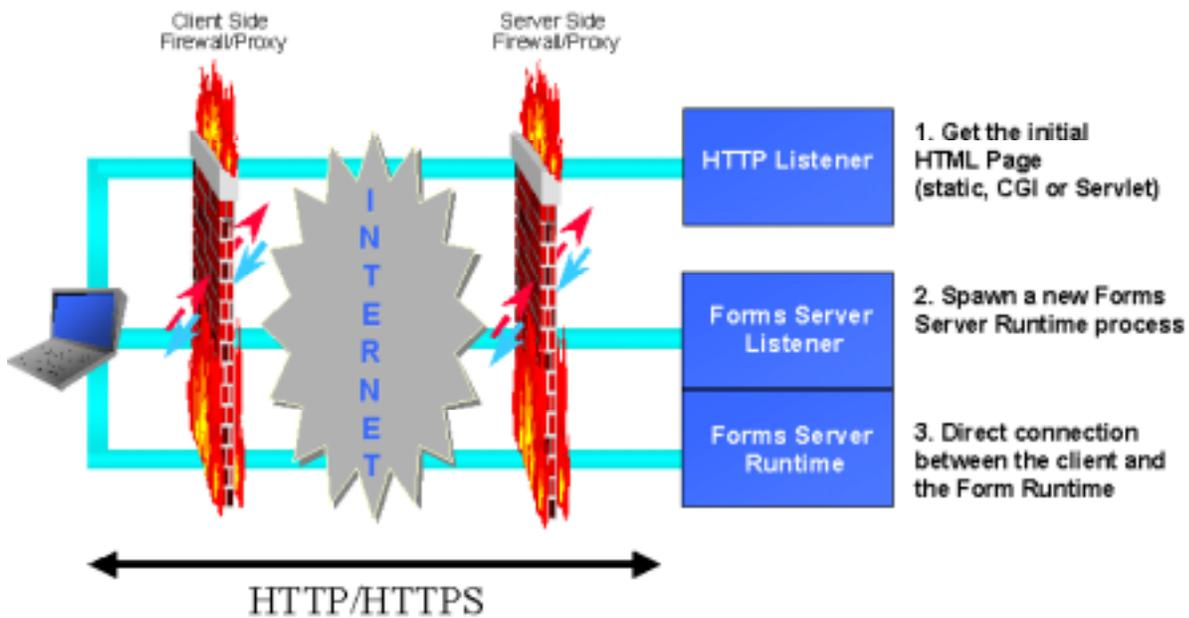
**Figure 1. Pre-Patch 4 Forms Server architecture for Internet deployment**
