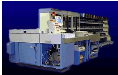
USPS Mail Processing Equipment (MPE) Scanner & Sorter
