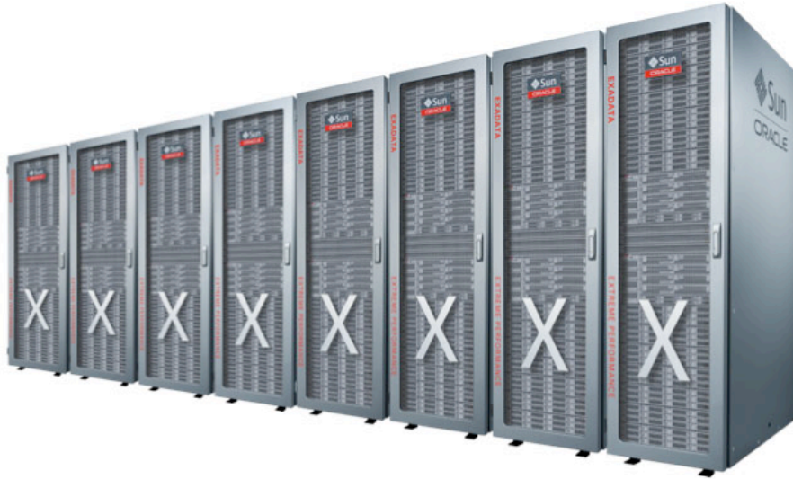
Figure 1 Eight connected Oracle Exadata Database Machine racks form a single system.
