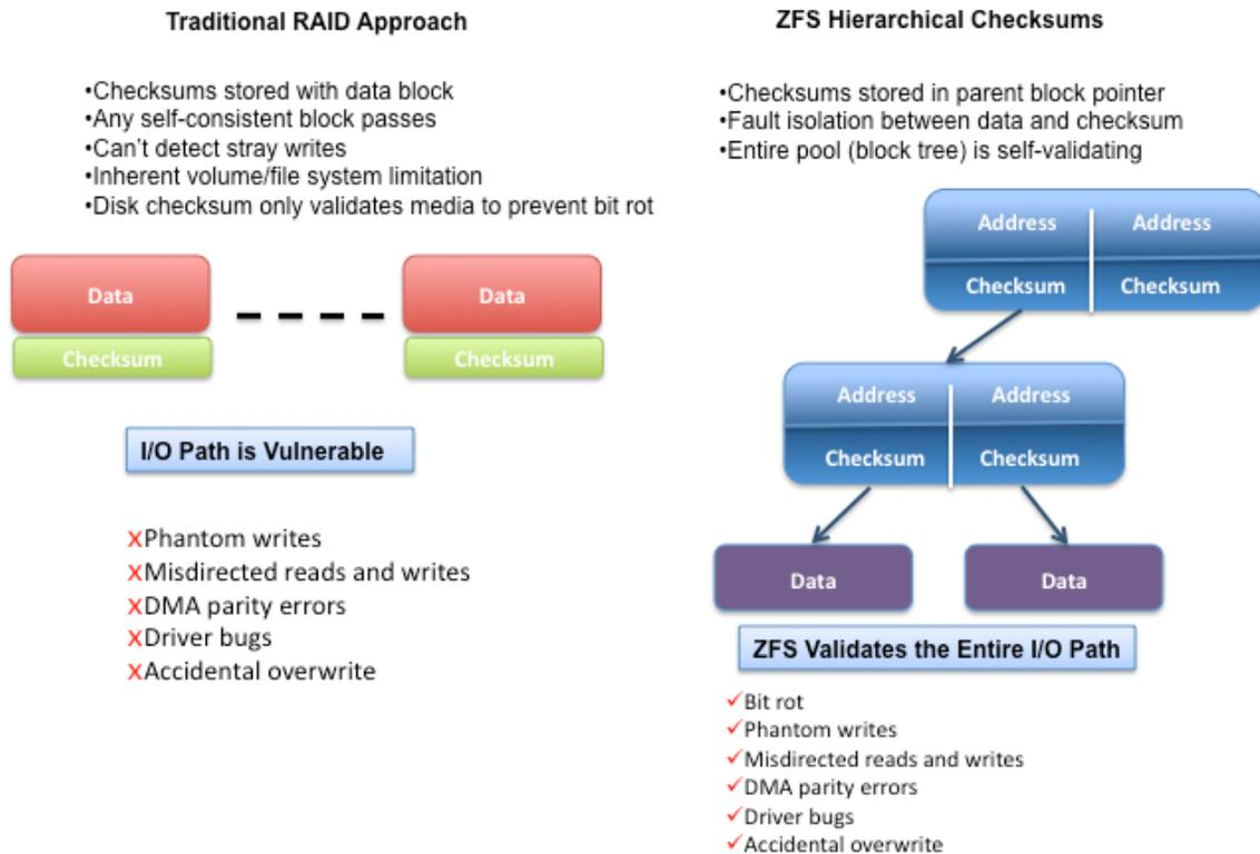
Figure 7: Description of ZFS hierarchical checksums versus traditional RAID approach.
