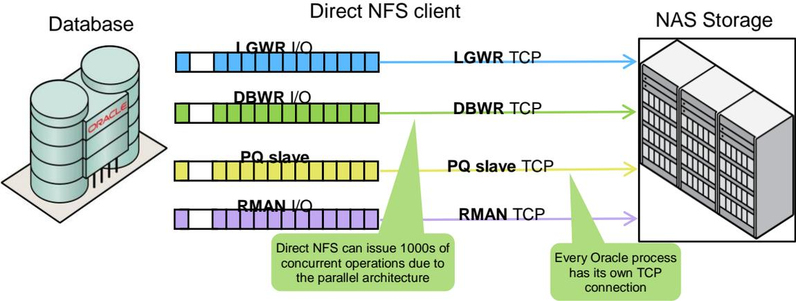
Figure 11: Architecture of a Direct NFS client
