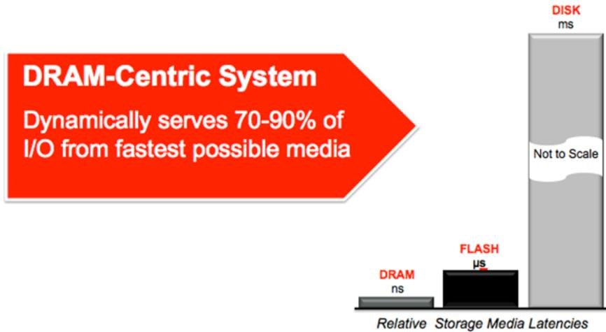
Figure 8: Illustration of the relative latencies of reads served from different media types.
