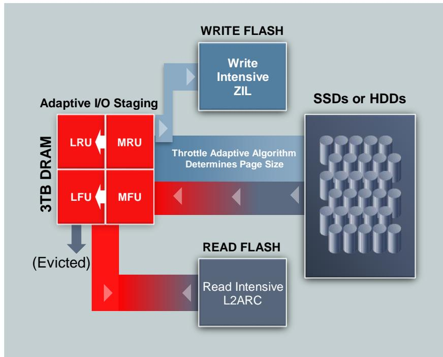
Figure 9: Graphical depiction of the Hybrid Storage Pool architecture that illustrates dynamic storage tiering.
