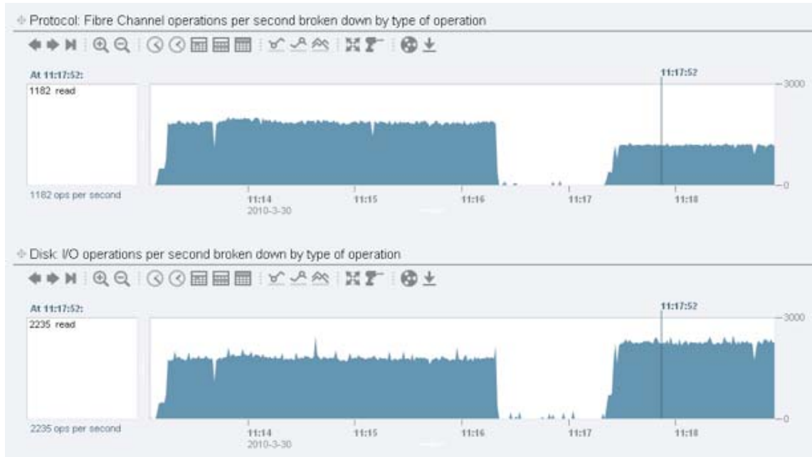
Figure 12. I/O displays for partition of EFI labeled LUN; start sectors 256 and 34 respectively
