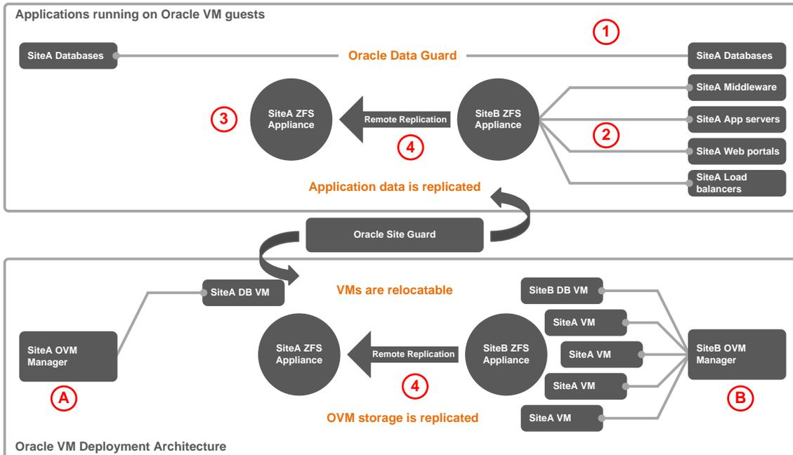
Figure 8: Conceptual look at how Oracle VM guests and applications are transitioned to alternate site by Oracle Site Guard
