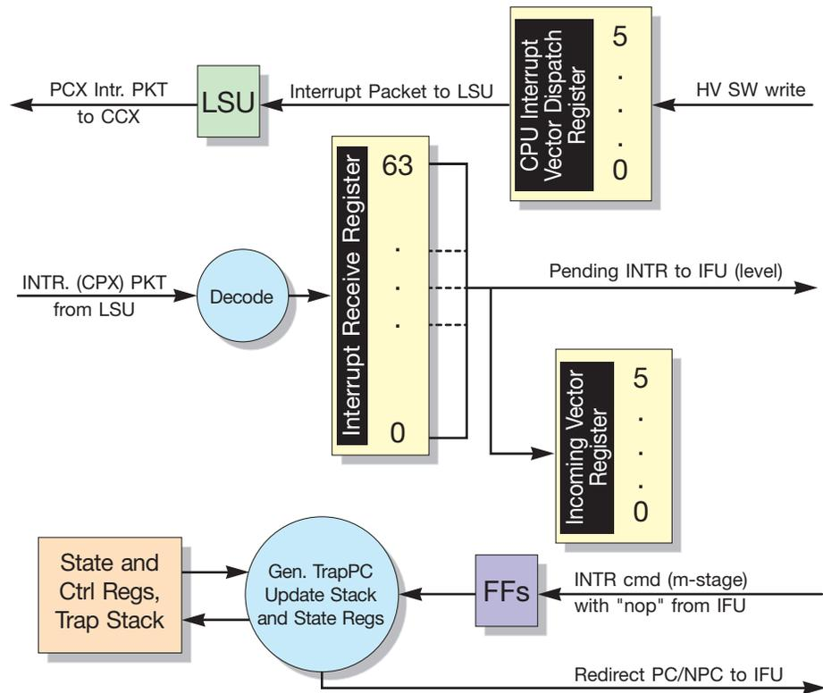
FIGURE 2-31 Flow of Hardware and Vector Interrupts
