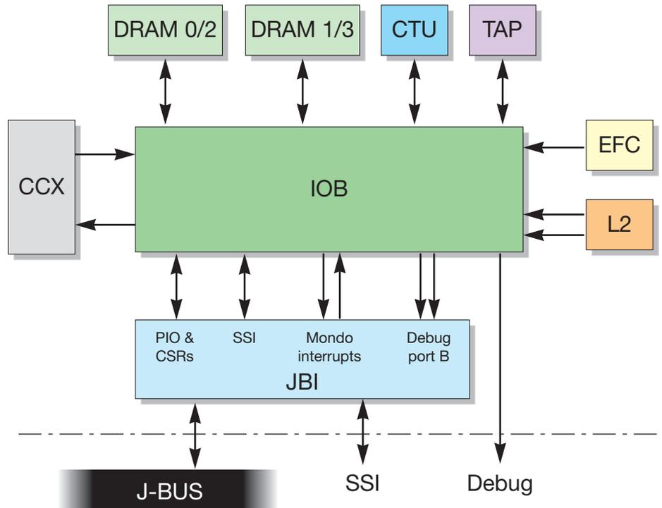
FIGURE 5-1 IOB Interfaces
