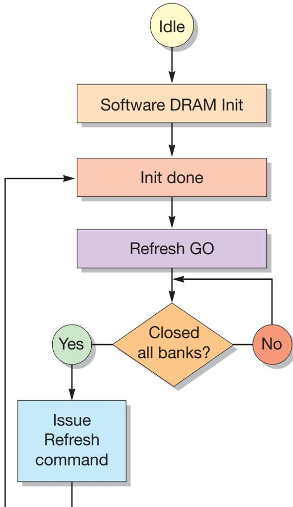
FIGURE 8-2 DDR-II DRAM Controller Top-Level State Diagram
