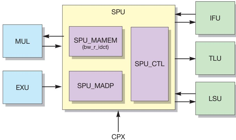
FIGURE 2-22 Data Flow of Modular Arithmetic Operations
