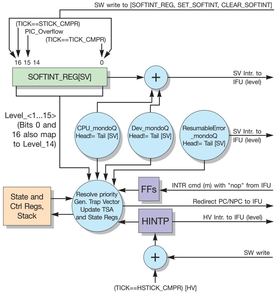
FIGURE 2-33 Flow of Software and Timer Interrupts
