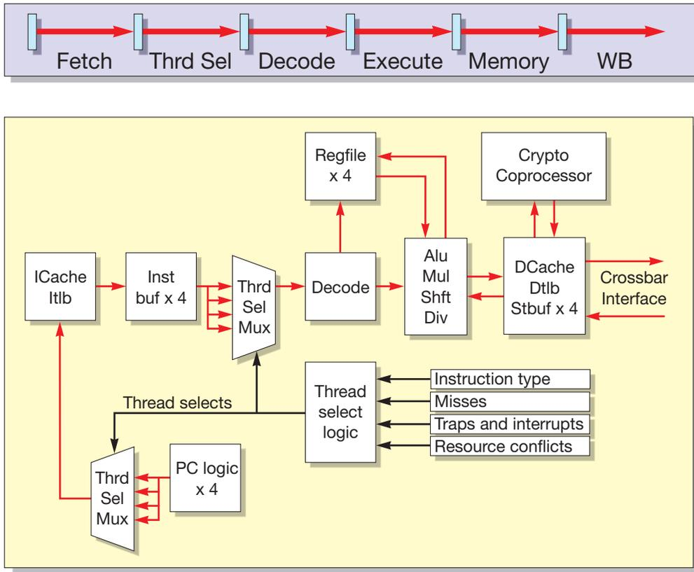
**FIGURE 2-4** SPARC Core Pipeline and Support Structures
