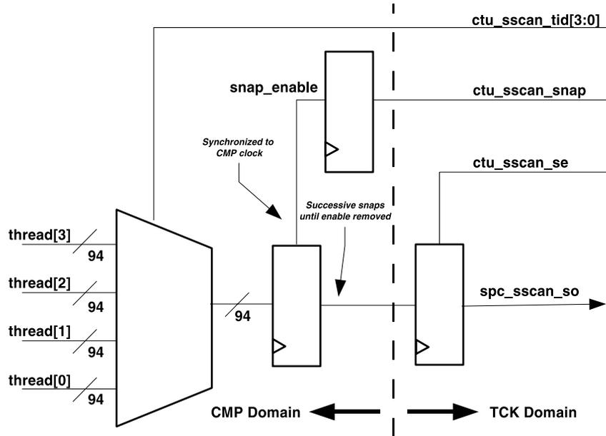
**FIGURE 2-37** SPARC Shadow Scan Chain
