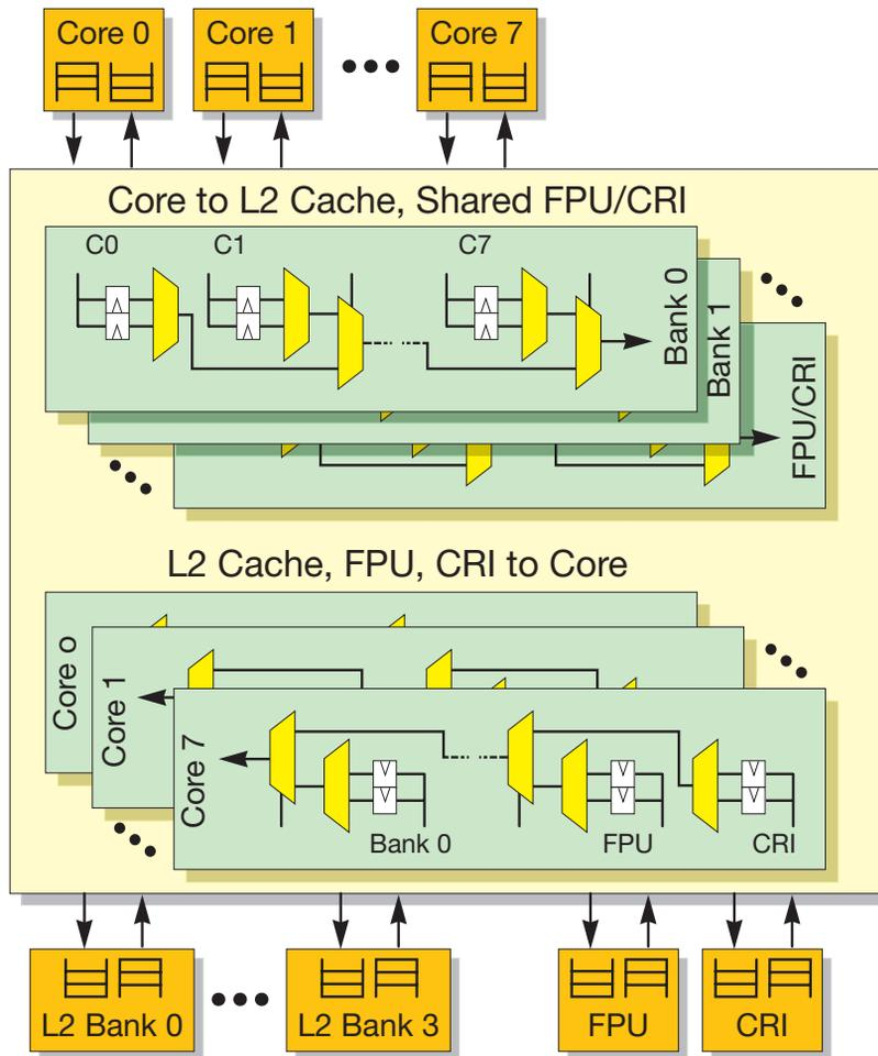
FIGURE 1-3 CCX Block Diagram
