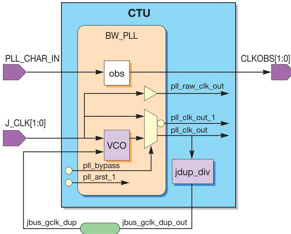
FIGURE 10-2 PLL Functional Block Diagram
