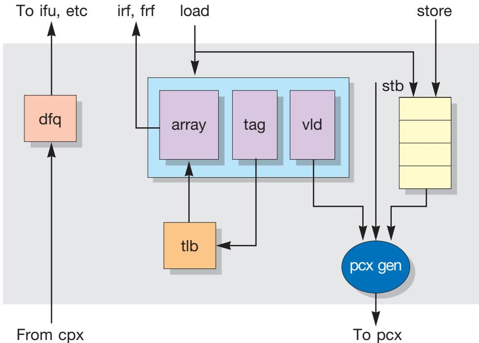
FIGURE 2-14 LSU Data Flow Concept
