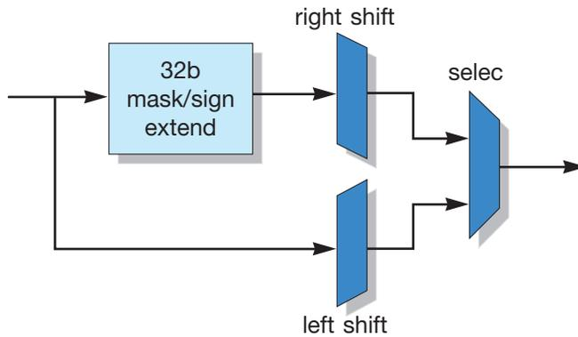
**FIGURE 2-16** Shifter Block Diagram
