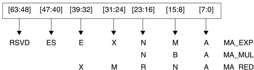
**FIGURE 2-21** Layout of MA\_ADDR Register Bit Fields
