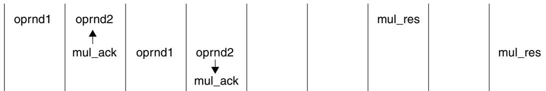
FIGURE 2-24 Multiply Function Result Generation Sequence Pipeline Diagram
