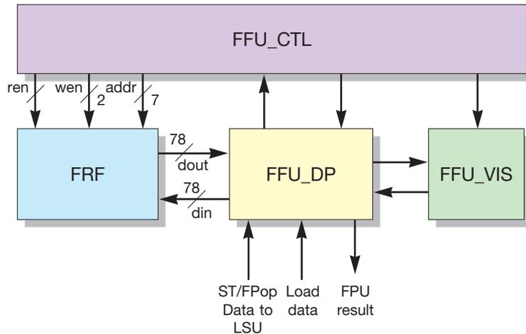
**FIGURE 2-19** Top-Level FFU Block Diagram
