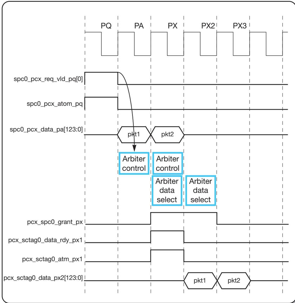
FIGURE 3-5 PCX Packet Transfer Timing – Two-Packet Request
