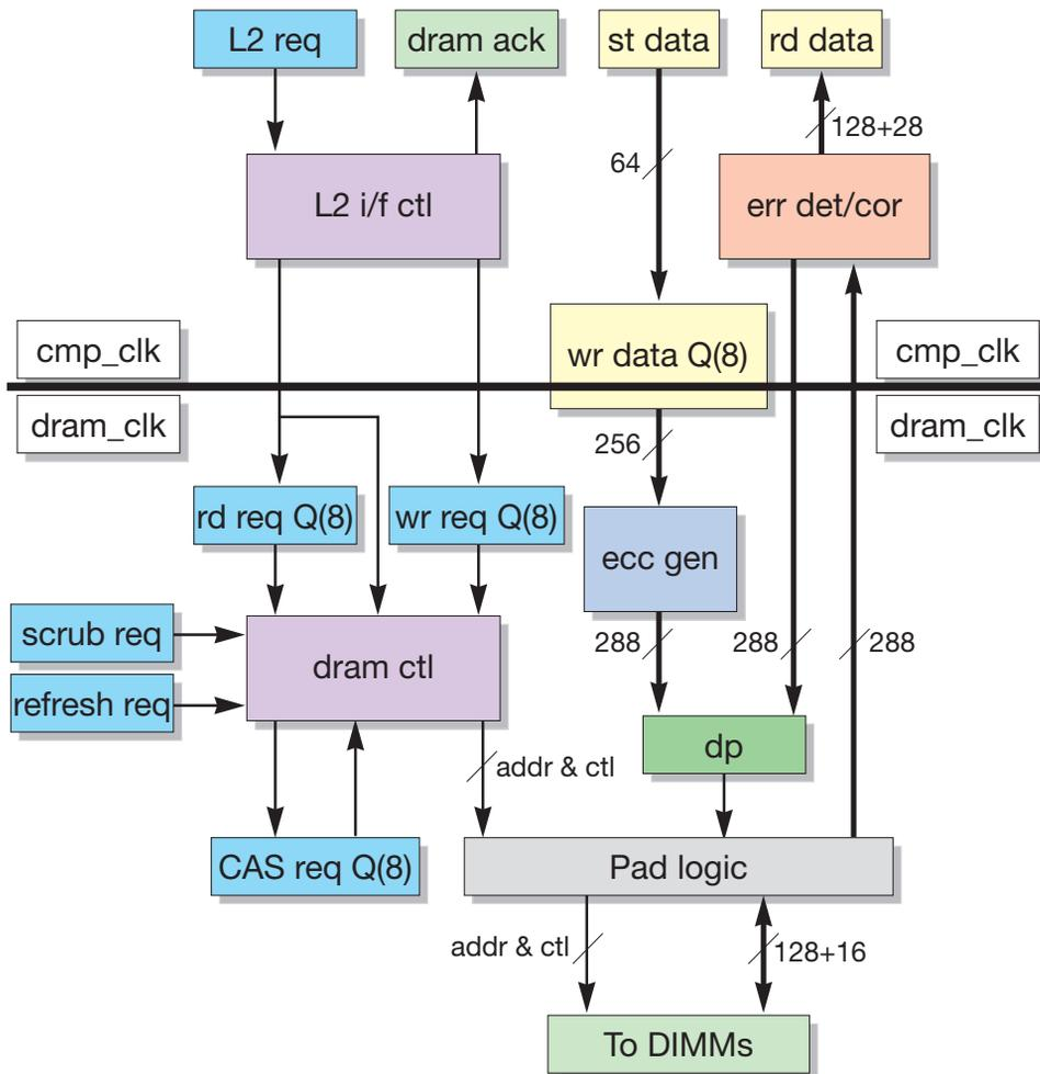
FIGURE 8-1 DDR-II DRAM Controller Functional Block Diagram
