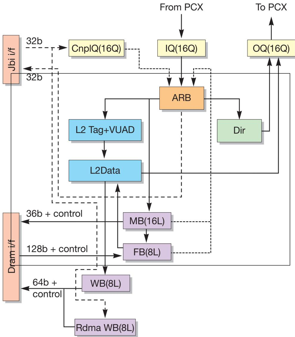
FIGURE 4-1 Flow Diagram and Interfaces for an L2-Cache Bank
