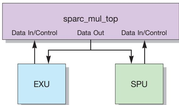
**FIGURE 2-20** Multiplexor (MUL) Block Diagram
