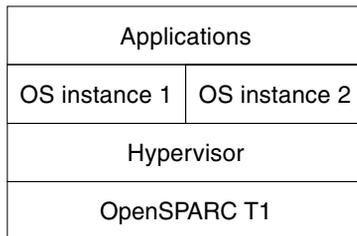
FIGURE 2-3 Virtualization of Software Layers
