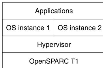
**FIGURE 2-26** Virtualization Diagram
