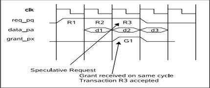
**FIGURE 3-9** Timing Diagram - Third Speculative request is rejected and resent later
