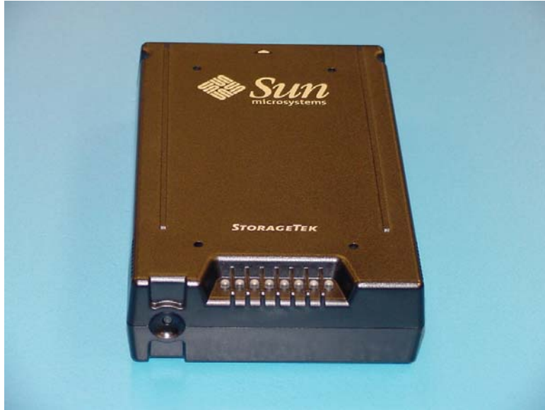
Figure 2 -- Front View of the Key Token. Recessed Reset Button shown on the left, 8-element LED Array centered
