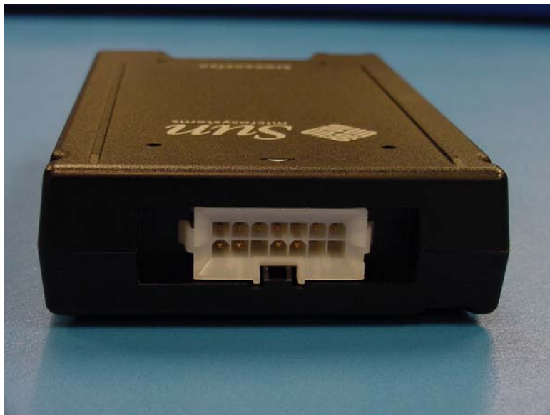
Figure 3 -- Rear View of the Key Token, 14-pin Connector. Pin allocation: 9 Ethernet port pins, 2 pins for DC PWR/GRD, 3 pins removed.
