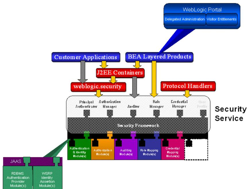
Notice in the figure above that WebLogic Portal adds some features to the underlying WebLogic Server security services. It includes its own authentication and identity assertion providers: RDBMS Authentication provider and Web Services for Remote Portlets (WSRP) Identity Assertion Provider modules that are used in conjunction with access to Portal Web objects.
