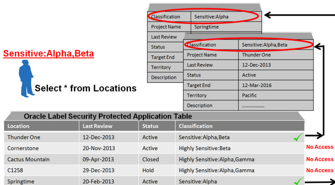
Figure 1. Oracle Label Security leverages user labels and data labels to control data access.
