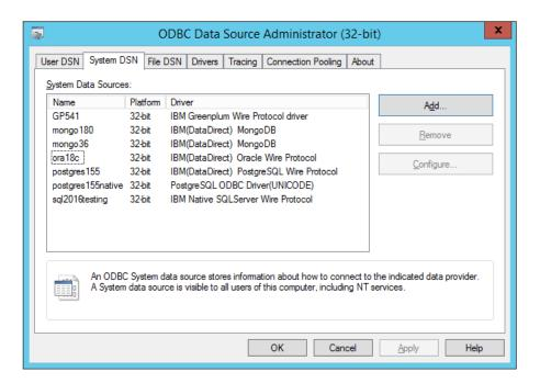
4. Click on Add to configure a new system DSN under the System DSN tab. Locate the DataDirect 8.0 Oracle Wire Protocol from the list of drivers presented to you and press finish.
