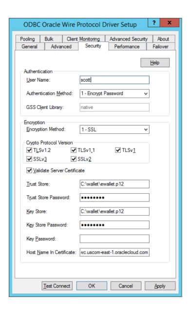
7. Test your connection by pressing the Test Connect button. Supply the database username and password to test the connection.
