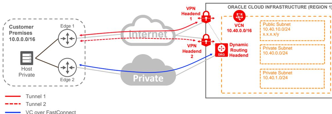
Figure 6. FastConnect Plus a Single VPN Connect Connection
