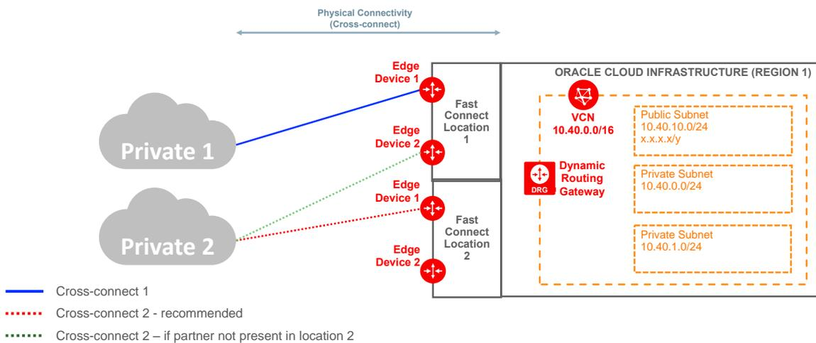
Figure 9. Physical Overview of an Oracle FastConnect Region
