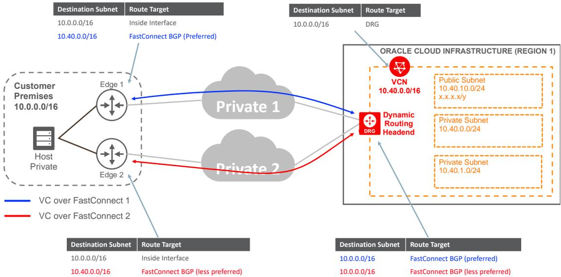
Figure 11. Redundant FastConnect—Routing
