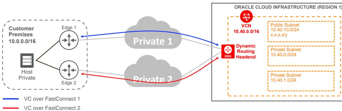
Figure 10. Redundant FastConnect
