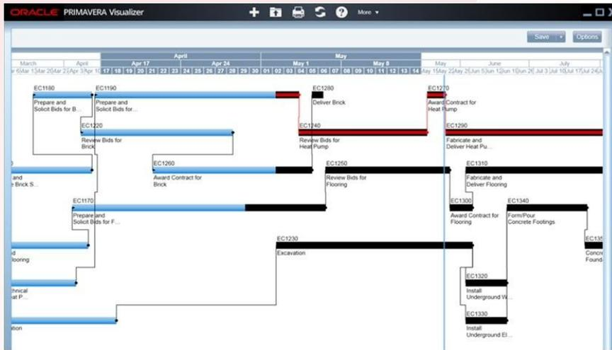
Figure 2. Time-scaled logic diagram with a zoomed timescale area showing relationships and critical activities.
