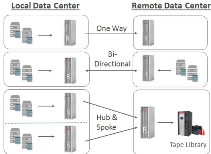
Figure 4. Recovery Appliance Backup Data Replication Topologies (Source: Oracle)
