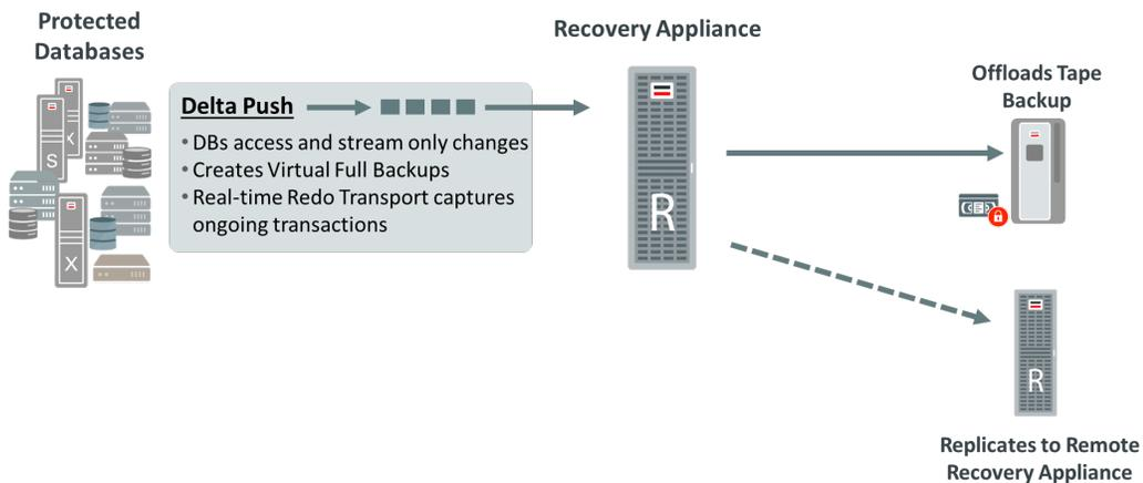
Figure 2. The Oracle Recovery Appliance Data Protection Environment showing Delta Push example. (Source: Oracle)
