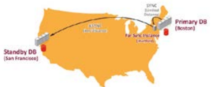
Figure 7: Active Data Guard Far Sync – High performance, zero data loss across large distance WAN
