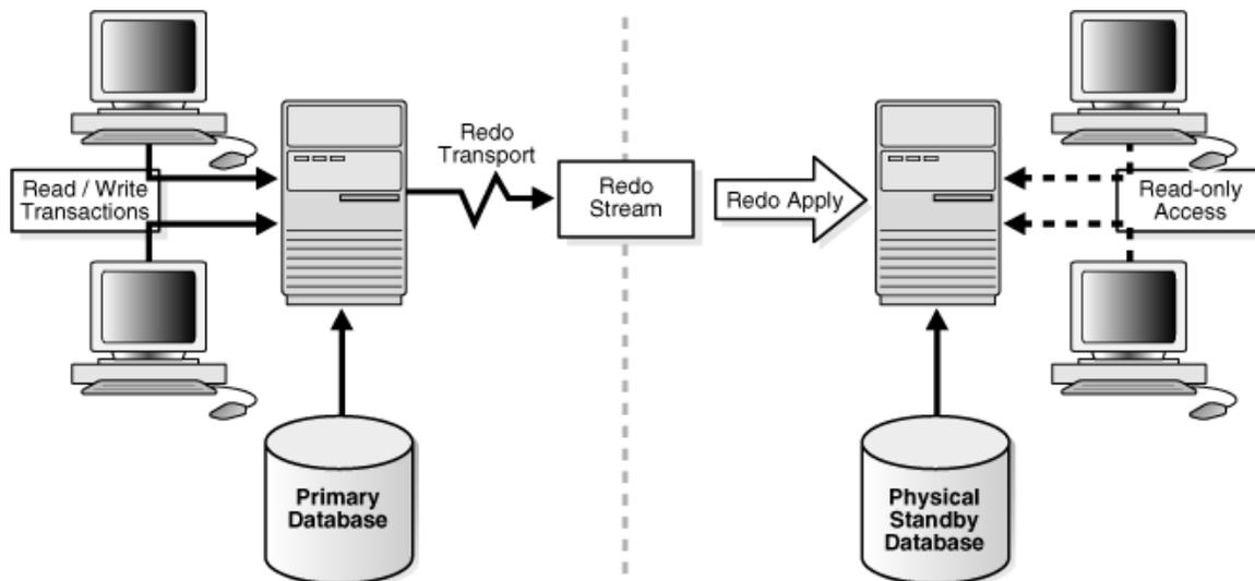
Figure 3: Automatic Updating of a Physical Standby Database
