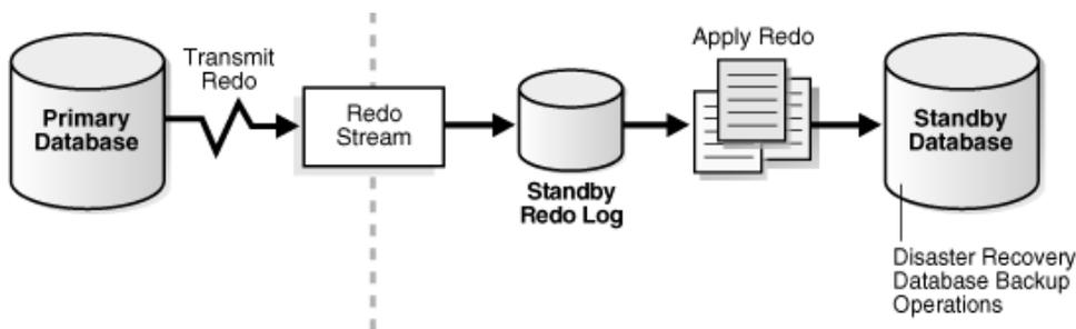
Figure 2: Typical Oracle Data Guard Configuration
