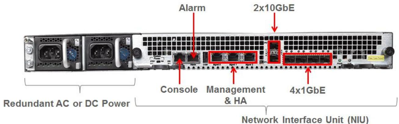
As seen in the above picture, the 4600 platform has a field replaceable 2 x 10 Gb/sec and 4 x 1 Gb/sec NIU. The NIU supports Enhanced Small Form factor pluggable (SFP+) for the two 10 Gb/sec Ethernet fiber ports and Small form factor pluggable (SFP) for the four 1 GbE ports. Plug the slot 0 port 4 (s0p4, bottom of the two 10GbE interfaces) interface into your outside (Internet facing)
